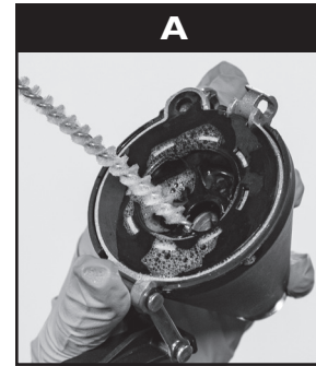
Remove Cleaning Brush from Case. Use mild soap and water to clean front cap/nozzle.
