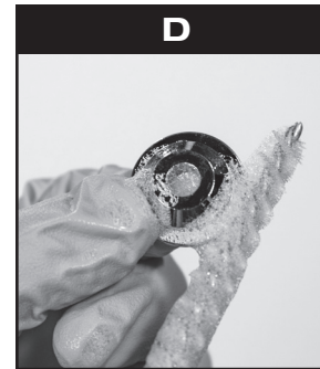
Rinse nozzle parts in water.
