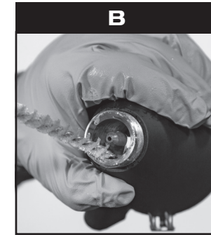
Remove Cleaning Brush from Case. Use mild soap and water to clean front cap/nozzle.
