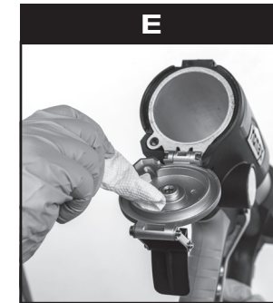
Use a damp cloth to clean Rear Gasket, Maintenance Valve, and sprayer body.
