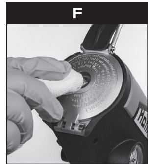
Use a damp cloth to clean Rear Gasket, Maintenance Valve, and sprayer body.
